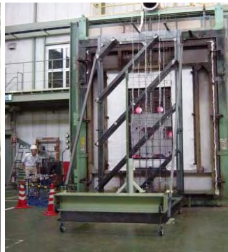
Fire test for Quake Resistance Facade
